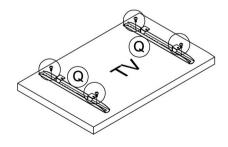
2. Secure the mounting bracket with a spacer if needed
